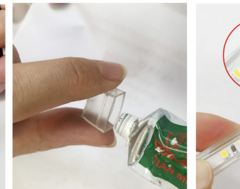
STEP 6 Tail plug filled with waterproof silicone
